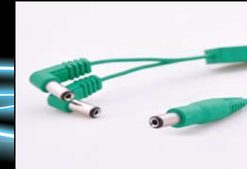
GREEN CURRENT DOUBLER CABLE Cable length 55 cm • 22" 2.1 - 2.1 mm • 1/16" DC Jack Combines 2 isolated outputs from a power supply into one DC plug and doubles the current.
