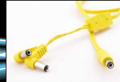
YELLOW VOLTAGE DOUBLER CABLE Cable length 55 cm • 22" 2.1 - 2.1 mm • 1/16" DC Jack Combines 2 isolated outputs from a power supply into one DC plug and doubles the voltage.
